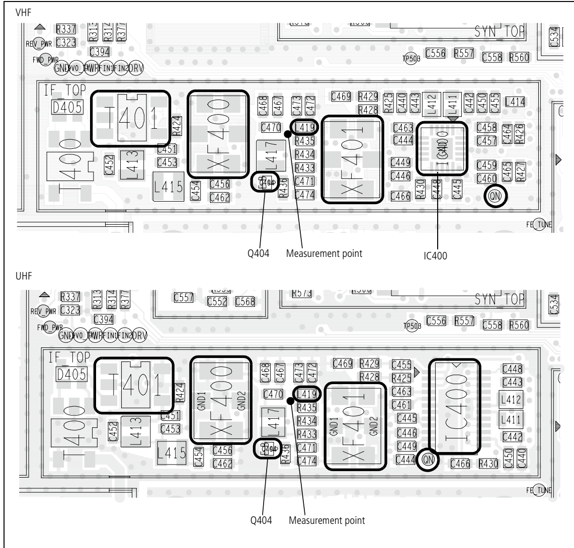
Figure 10.1 Receiver circuitry under the IF TOP can (top side)
